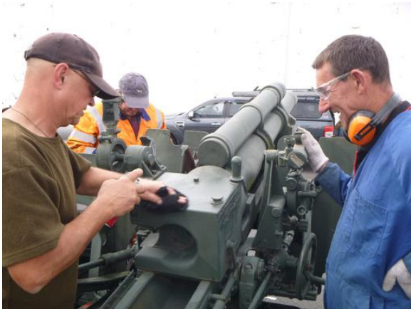
Removing gnarly welds around the breechblock and elevation gear and related components..
