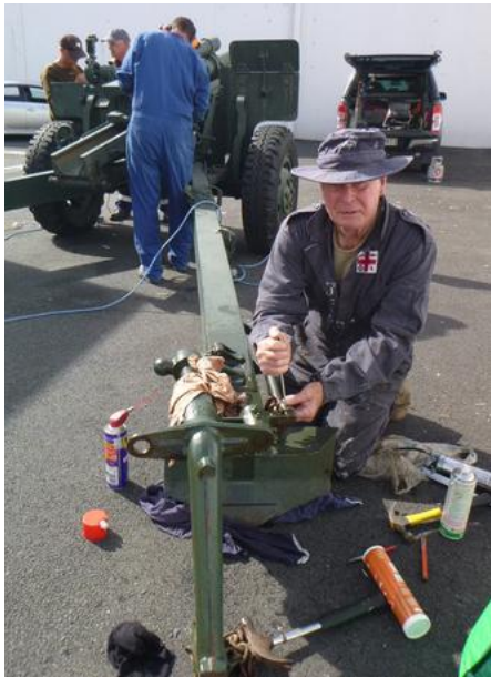
Removing gnarly welds around the breechblock and elevation gear and related components..
